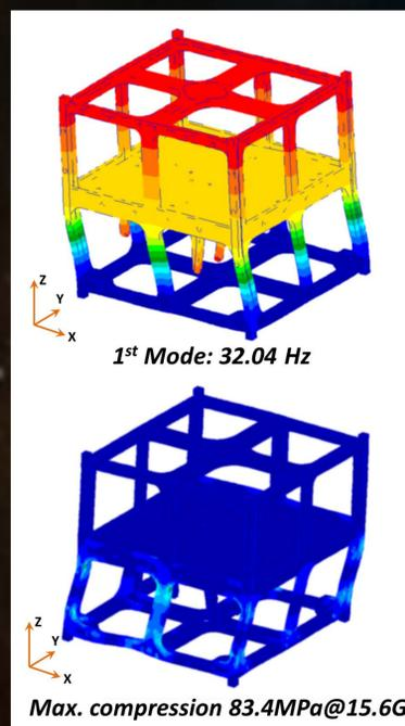
Figure 3: Mechanical analysis.
