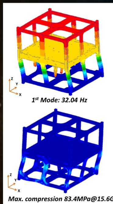
Figure 3: Mechanical analysis.
