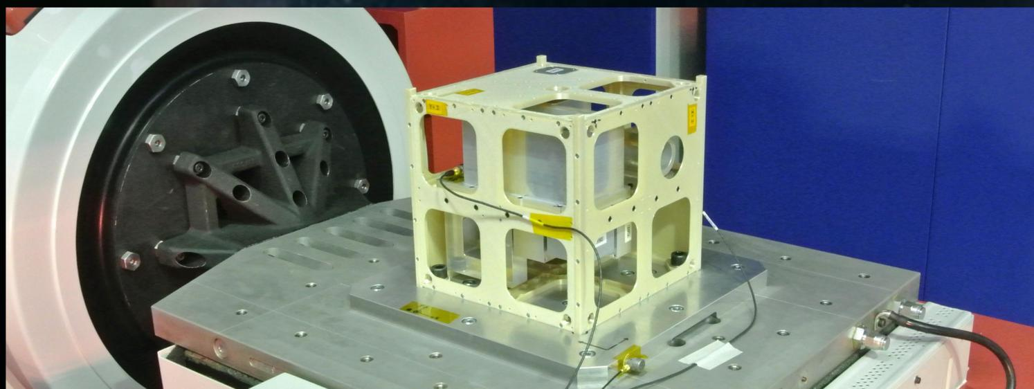
Figure 1: Structural model with 3D printed on top of the shaker during the mechanical qualification tests.
