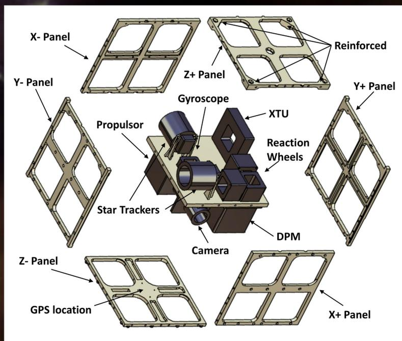
Figure 2: New structural design.
