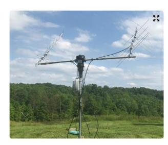
Yaesu G-5500 with M2 cross yagi antennas and S-band parabolic dish
