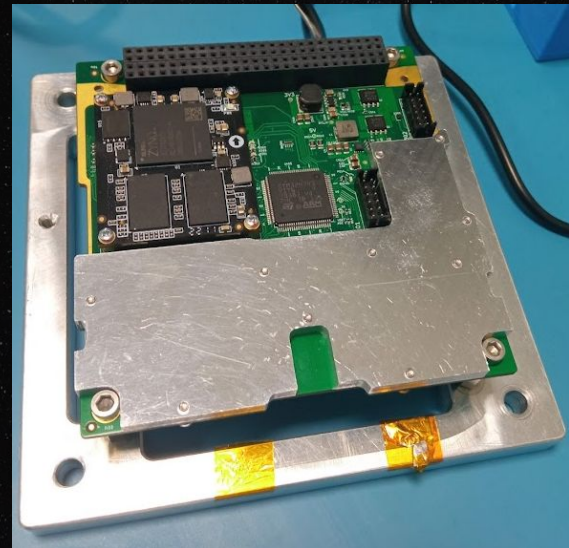
Manufactured COMMS Board
