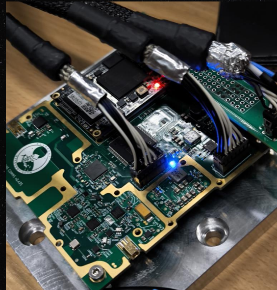
Manufactured COMMS Board during functional tests
